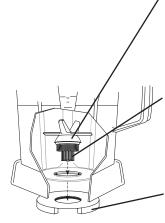
Blade Agitator Assembly. Use caution when handling the blade; it is sharp. When inserting the blade assembly through the container bottom, align the flat sides. Gravity holds it in place while the retainer nut is tightened. Do not attempt to disassemble this part.
